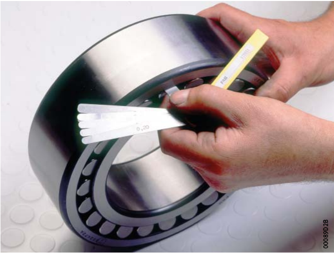
Figure 11 Measuring the radial internal clearance
